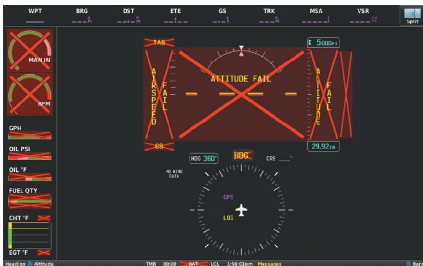
G3X Touch System Failure Annunciations
