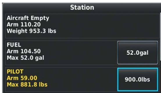
Loading Limit Exceeded
